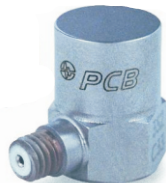
352C03- Single Axis 10 mV/g, 500 g pk 5.8 gm
