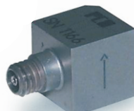
333B30 - Single Axis 100 mV/g, 50 g pk 4.0 gm
