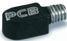
352C23-Single Axis 5 mV/g, 1000 g pk 0.2 gm
