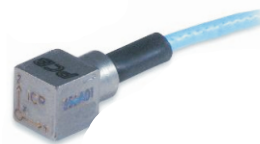
356A01- Triaxial 5 mV/g, 1000 g pk 1.0 gm
